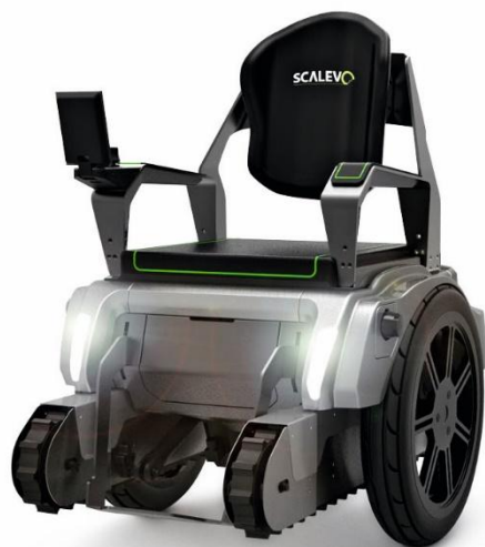
A 3D model of the Scalevo wheelchair. Image ©Scalevo
