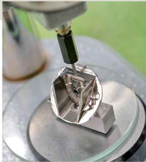
The individual parts of the Bone Anchored Port are precisely measured; the machined metal surface cannot contain a single scratch.
